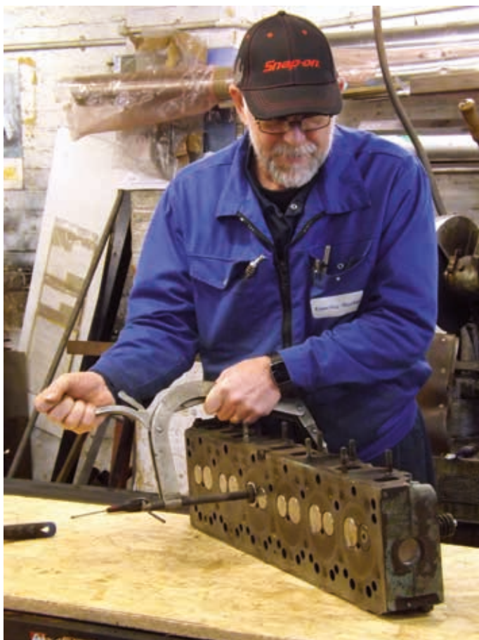
Ford cylinder head repair
