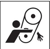
Never operate the engine without covers on the moving parts.
